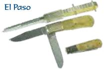
Traditional styling of our El Paso Slip Joint folder is complimented with filework on the mirror polished AUS-8A Stainless Steel blades and the back splines with added features of the embossed bolsters, Brass liners and Nickel Silver pins. 6-3/16" overall open, 3-1/2" x 1" when closed. 2-3/8" cutting edge. Minimum handle material size: 1" x 2-3/8" x .135". TD47 and TD40 drills.
