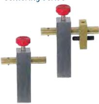
Use this handy tool to scribe the center lines as a guide for grinding knife blades. Designed for accuracy, this scribe can be adjusted from 0-1/2". Adjusts 1/32" per revolution using fine adjustment screw. Replaceable carbide tip marks even the hardest knife steel.
