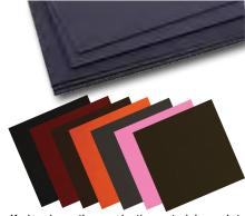
Kydex is a thermoplastic material used to make formed sheaths for your knives. It is cut to shape, formed by use of a heat gun then held firmly together with rivets, eyelets, or glue. With a little practice, you can make a protective sheath in minutes. Protect tools, kitchen cutlery, and many other items using this easily formed material. Also a great Basic instructions are holster material. Basic i included. Kydex is 12" x 12".
