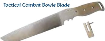
Cut your way through brush, limbs and most any deep adventure situation with this durable addition to our Bowie blades. CPM 3V flat ground steel offers great impact resistance. This allows maximum resistance to breakage and chipping. Nickel Silver guard and pin included. Cryogenically treated and razor sharp. Overall length 13 1/4", blade is 8 1/4" x 1 1/5" wide, 3/16" thick. Handle Holes 3/16".
