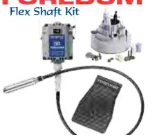
Features a 1/6 hp reversible ball bearing motor. 0-18,000 rpm. Hang up model has a 39" flex shaft. Complete with electronic foot control, #FH30 handpiece, chuck key, shaft grease plus a 54 pc. accessory kit. 110-130 v. Maintenance kit includes inner flex shaft, pair motor brushes, grease.
