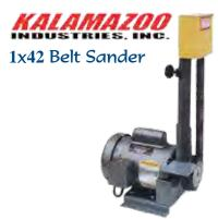
1/3 HP motor, 1PH, 1725 RPM. 4" contact wheel, tilt table. Vertical sander. 1800 SFPM. Platen can not be removed. Actual shipping charges apply. Use 1" x 42" belts.
