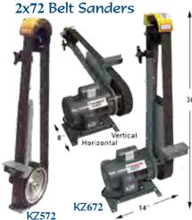
With or without 1/2 HP motor, Kalamazoo sander vertical or horizontal. 2" x 72" belt, tilt table, 8" serrated contact wheel, removable platen.--KZ572 is belt driven with supplied pulley V-belt. WT 24 lbs. --KZ672 is 3450 RPM. WT 80 lbs. Both use 2" x 72" sanding belts. Actual shipping charges apply.
