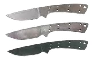
Pattern 37 flat ground blades are cryogenically processed during heat treating for optimal edge holding capability. Overall length 6 5/8", Blade Length 2 5/8", Blade Width 7/8", Blade Thickness 1/8". Bolster holes 1/8", Handle Holes 1/8", Thong Hole 3/16". Available in D2, CPMS 30V, 440C, 1095 and Damascus steels. Offered in peened or satin finish. Available leather sheath KT370.
