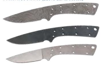
Pattern 36 blades are cryogenically processed during heat treating for optimal edge holding capability. Overall length 7 5/8", Blade Length 3", Blade Width 1", Blade Thickness 1/8". Bolster holes 1/8", Handle Holes 1/8", Thong Hole 1/4". Flat ground. Available in D2, CPMS 30V, 440C, 1095 and Damascus steels. Offered in peened or satin finish. Available leather sheath KT360.
