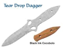
Designed stainless steel dagger blade with a bead blast finish. Overall length is 10", 4" blade, 1 1/8" wide and 1/8" thick. Built in guard is 2" wide. Tang holes are 7/32".
