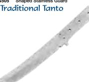
Traditional Tanto style blade, the upswept tip and wide handle make this blade stand a cut above. Pre-drilled with three 3/16" tang holes and two 3/32" bolster holes. 12 1/2" overall, the blade is 6 1/2" x 1 3/16" wide and 3/16" thick.
