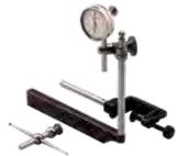
Sensitive, reliable and easy-to-read. With its three hardened contact points, the Universal Dial Test Indicator adjusts to any angle. Graduated in .001 dial reads 0-100 with a range of .200. Set comes with points C, D, and E. Plus four attachments (a) clamp with 5/16" rod, (b) tool post holder with 5/16" rod, (c) snug complete for attaching (a) or (b) to dial test indicator, and (e) hole attachment. All in a fitted case. Made in
