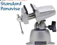
The Standard PanaVise gives you a complete range of adjustments to suit your needs. With rotation through 360° and 180° tilt, PanaVise provides the perfect angle on any job. This vise opens to 2 1/4" with 15/16" throat. 2 1/2" nylon jaws can withstand continuous heat to 200°F. Head removes easily from base for additional use when grinding, polishing or drilling those hard to grip pieces.
