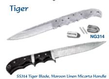
This satin finished premium 8-A stainless steel hollow ground blade is easy to hold and practical to use. Overall length is 9-1/2", blade is 4-1/2" x 1" x 5/32" thick. A very stylish trend of two contrasting handle materials can easily be accomplished with the double slots for double guards. Slots are .270" wide and 5/32" thick and requires 3mm guard and handle pins. and 7/32" thong hole. Available sheath KT111.
