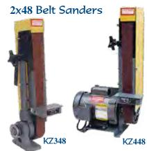
With or without 1/2 HP motor, 1PH, 3450 RPM. Each come with 5" contact wheel, tilt table and removable platen. Full hinged guard for quick belt change. Can be mounted vertical or horizontal. KZ448 runs 3450 SFPM. KZ348 is belt driven supplied pulley V-belt. Both use 2" x 48" sanding belts. Actual shipping charges
