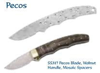
The Pecos is a very small ultra mirror polished 8A stainless steel skinner blade with a tapered tang. Drilled with twelve 2mm holes around blade edge, three 3mm holes in the center, one 2.5mm hole for a custom bolster if desired and a 3/16" thong hole. Overall length is 6", blade is 1-7/8" long x 7/8" wide x 1/8" thick. Available sheath KT106.
