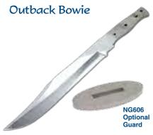
15" overall, 9" blade 1.72" wide. Hollow ground from 3/16" 440-C stainless blade stock. Handle is designed for balance and ease in handling. Double guard is available in brass or nickel silver. Brass guard is 3/16" x 1" x 4", nickel silver guard is 1/4" x 1" x 4". Use mini corby rivets or 5/32" pins. Kit includes blade, CP935 brass guard, pins and handle material. Available sheath KT485.
