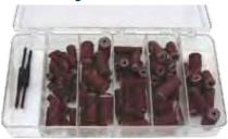
These resin-bond rolls are 1" in length. Mandrel is available in 1/8" or 1/4" shank. Recommended safe speed is 15,000 rpm. Kit contains 60 resin bond cartridge rolls plus two 1/8" mandrels. Stored in a handy plastic box. For wood or metal, like sandpaper. Roll out to desired size.
