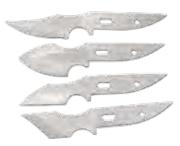
Four piece set of the most used wood carving blades. We added this set for the woodworkers who want to make their own handle for a custom feel. Sold in sets only. 440-C Stainless. Overall length of each 4 1/2" - 5". Slot wood to proper angle to insert blade and fasten with 1/8" pins.
