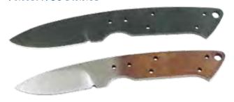
Pattern 38 blades are cryogenically processed during heat treating and flat ground for optimal edge holding capability. Overall length 7", Blade Length 2 1/2", Blade Width 15/16", Blade Thickness 5/32". Bolster holes 1/8", Handle Holes 1/8", Thong Hole 1/4". Flat ground. Available in D2, CPMS 30V, 1095 and Damascus steels. Offered in peened or satin finish. Available sheath KT380.
