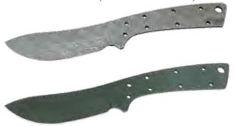
Pattern 32 blades are cryogenically processed during heat treating for optimal edge holding capability. Flat Ground. Overall length 7 5/8", Blade Length 3 1/8", Blade Width 1", Blade Thickness 1/8". Bolster holes 1/8", Handle Holes 1/8", Thong Hole 1/4". Available in D2, 154CM, 440C, 1095 and Damascus steels. Offered in peened or satin finish. Available sheath KT320.
