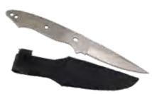
False top edge and thumb notches on this stainless steel blade. Kit contains three 3/16" brass pins, handle material, blade and Nylon sheath. Overall length 8-3/4", blade is 3-1/2" x 7/8" wide x .108" thick.
