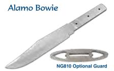
Our most popular Bowie Blade is made from 440C Stainless steel. The fame is in the name. This Bowie style blade whose design became a legend at the Alamo is a must for every knife collector. 13" overall length, blade is 8" x 1 1/2" x 5/32" thick. Three 5/32" pin holes. The #CP475 preslotted brass guard is 4" long 3/4" wide and 1/4" thick. Our Alamo Bowie kit includes the blade, CP475 pre-slotted brass guard, brass handle pins and handle material. Available sheath KT128.
