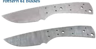
Pattern 61 flat ground blades are cryogenically processed during heat treating for optimal edge holding capability. Overall length 7 3/4", Blade Length 3 1/4", Blade Width 1 1/4", Blade Thickness 9/64" (.140"). Bolster holes 3/32", Handle Holes 3/32" and 3/16", Thong Hole 1/4". Available in D2, 440C and Damascus steels. Offered in peened or satin finish. Available sheath KT610.
