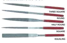
Fast cutting diamond files for ultra hard materials. 7 1/8" overall. Equalling file is 3/8" wide, 3/32" thick. Square is 3/16" wide. Half round cuts flat on bottom and is 3/8" wide. Round is 3/16" diameter. Three Square is 1/4". All sizes are approximate.
