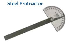
Preferred by machinists for setting bevels, measuring, and transferring angles. Made of ground stainless steel. Graduations from 0 to 180° in opposite directions. 3 3/8" x 2" head. 6" adjustable protractor arm locks into desired position with knurled thumb nut.
