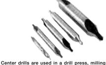
machine or lathe to start the hole to be drilled. The large body diameter and small drill size make them extremely rigid, thus eliminating any flex or 'walk' you will experience with other drills. Use to start the hole and to drill 'centers' on stock to be turned in a lathe.
