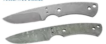
Pattern 31 flat ground blades are cryogenically processed during heat treating for optimal edge holding capability. Overall length 7 5/8", Blade Length 3", Blade Width 1 1/8", Blade Thickness 5/32". Bolster holes 1/8", Handle Holes 1/4", Thong Hole 1/4". Available in D2, 154CM, 1095 and Damascus steels. Offered in peened or satin finish. Available sheath KT310.
